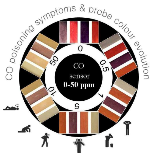
Figure 5.2. Scheme of the colour evolution of the colorimetric probes upon presence of increasing concentrations of CO.
