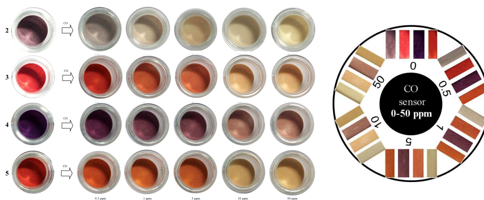
Figure 6. Sensing array of probes 2-5 for CO detection in air showing naked eye colour changes upon exposure of 0.5, 1, 5, 10 and 50 ppm CO.
