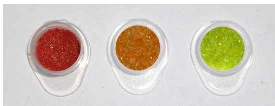
Figure S1. From left to right: color of ruthenium compound 1 , silica-adsorbed 1 , and the silica-adsorbed solid upon reaction with CO (to form 2 ).
