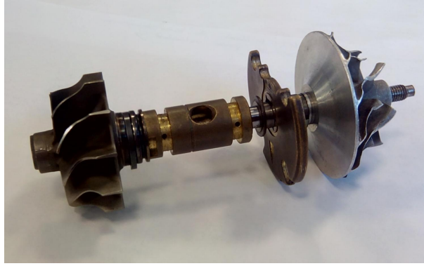
Figure 2.2: Turbocharger bearings. The radial bearings are visible as well as the axial bearing washers. The oil seals are also present
