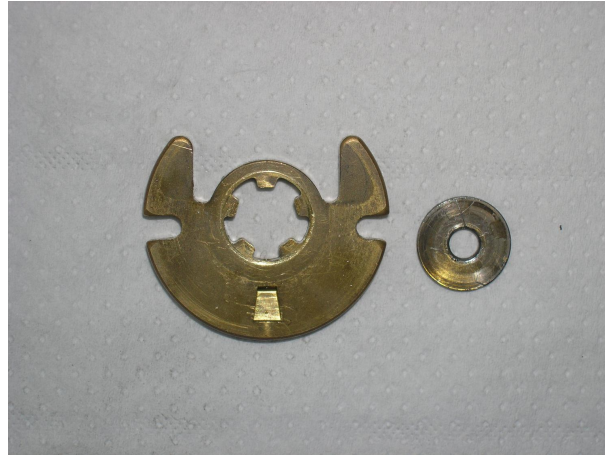
Figure 6.37: Damaged thrust bearing washers after high oil temperature experiments
