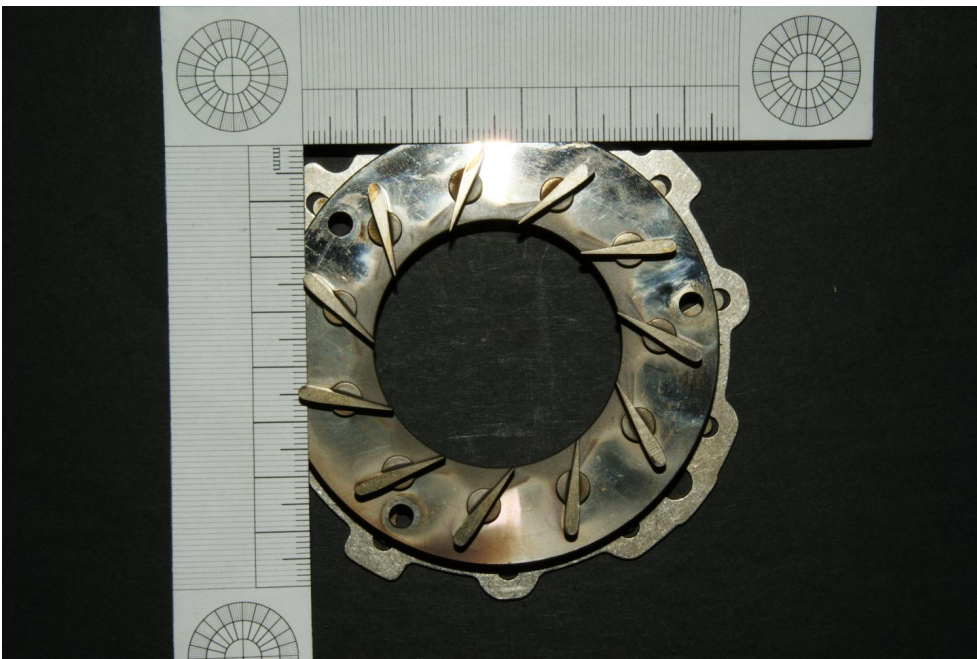
Figure 6.14: The turbine stator
