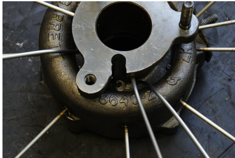
Figure 3.15: Turbine instrumented for internal pressure characterisation
