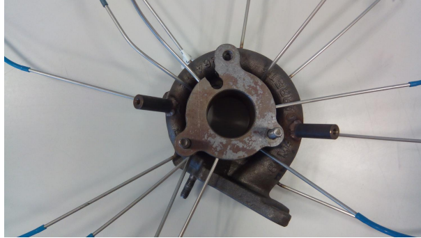
Figure 3.30: Fourth turbocharger, instantaneous pressure probes location
