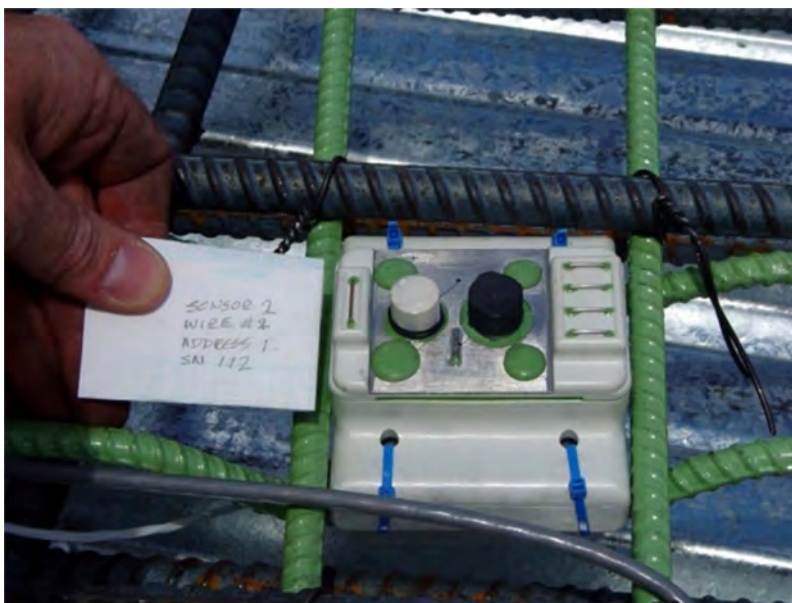
Fig. 2.1 Multisensor VTI ECI-1. Office of testing and technology services corrosion technology branch. California
