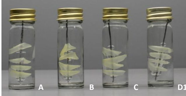
Figure 4.6. Resistance of gliadin film cross-linked with 5% of cinnamaldehyde after 10 days of contact at 40 °C with several food simulants.
