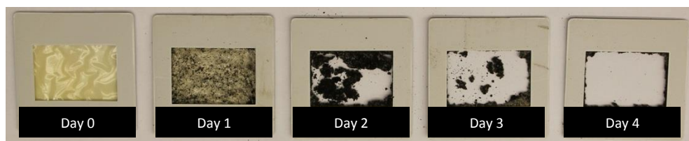
Figure 6.2. Qualitative view of disintegration of gliadin film G5C_pH2 exposed to composting conditions.
