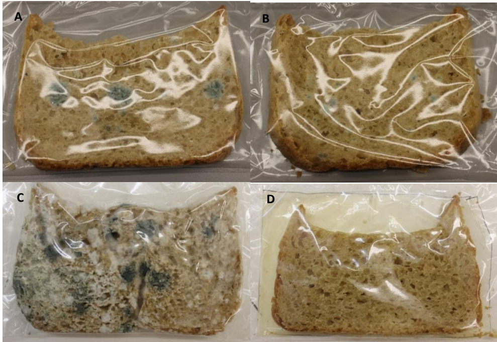
Figure 5.3. Growth of inoculated Penicillium expansum and fungi naturally present in (A) inoculated bread in control packaging after 14 days, (B) uninoculated bread in control packaging after 14 days, (C) uninoculated bread in control packaging after 1 month, and (D) inoculated bread in active packaging after 1 month (similar to uninoculated bread with active packaging after 1 month, results not shown).
