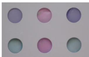
Figure 7. The polyethylene oxide membranes of 1 (top) and 2 (bottom) in the absence and presence DCNP (30 ppm) and HCl (50 ppm) vapors (from left to right).
