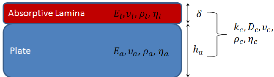
Figure 3.2: Scheme of a binary system composed of an absorbing layer (thickness \delta ) placed on the top of the plate (thickness h_a ). Each layer has its own elastic parameters that combine to produce a composite material (thickness h_c ), with new elastic parameters.
