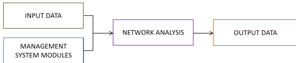
FIGURE 1. Modules in a PMS used to evaluate the suitability of maintenance programs at the network level
