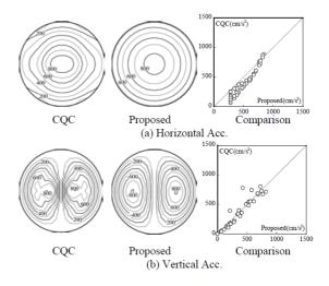
Figure.4. Acceleration Distributions in Dome
