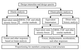
Figure 1. Design flow for member proportioning [1]
