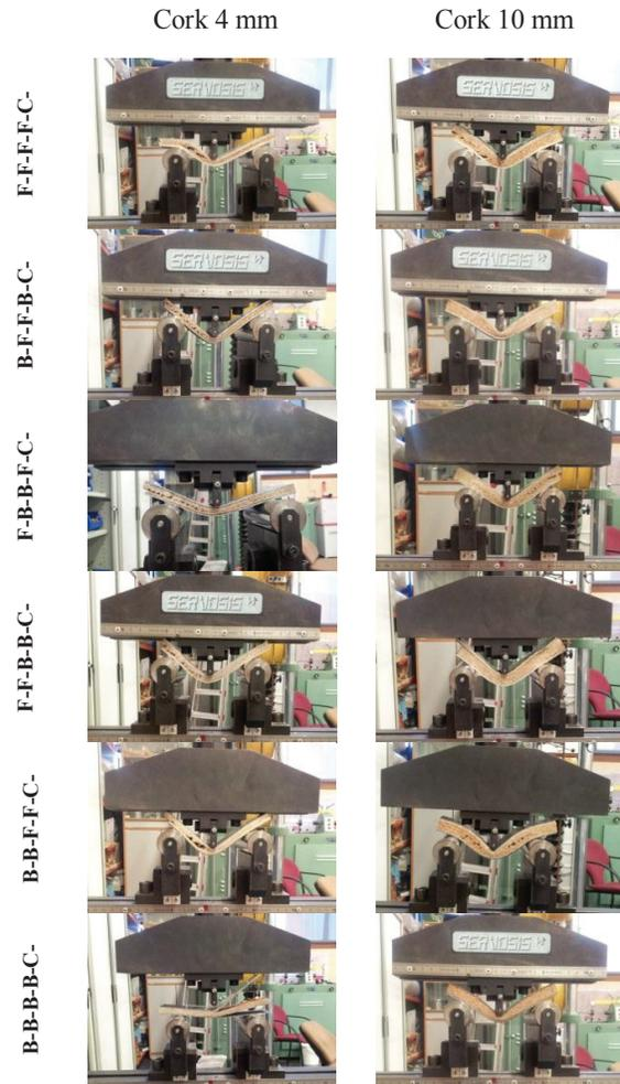
**Figure 5** – Images of flexural test of sandwich panels with different cork thickness and flax-basalt stacking sequence.
