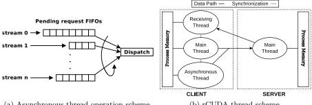
(a) Asynchronous thread operation scheme.
