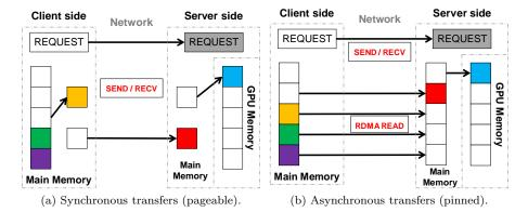
Figure 5: IBV pipeline support in IBV communications module.
