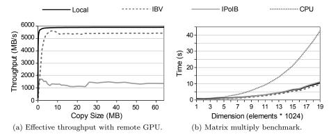
Figure 7: Remote GPU throughput and matrix multiply benchmarks.
