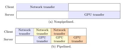
Figure 3: Transfer to remote GPU in nonpipelined and pipelined modes.
