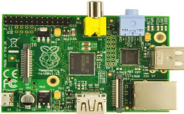
Figura 2.6 Raspberry Pi Model B
