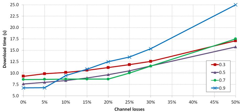
Fig. 20 Evaluation of the code rate of LDPC Staircase, with 3000-packet size and transmission rate=5 Mb/s
