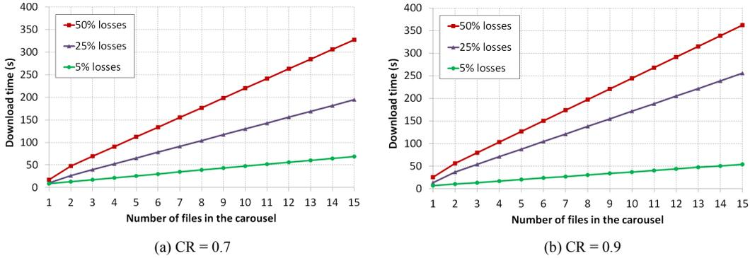
**Fig. 21** Evaluation of the number of files in the carousel, with files of 3000-packet size, coded with LDPC Staircase and transmission rate=5 Mb/s
