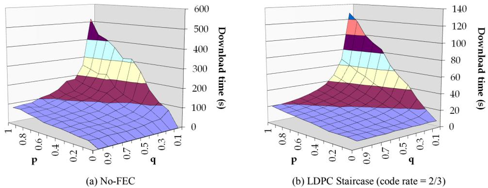
**Fig. 19** Download time depending on coding, with 3000-packet size and transmission rate=5 Mb/s
