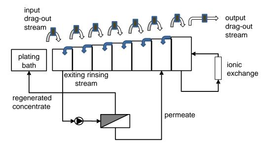
Figure 2. Rinsing process with RO regeneration
