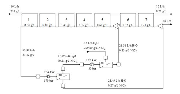
Figure 6. Simulation results for a two-stage configuration
