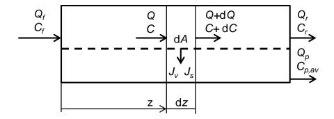
Figure 1. Scheme of the module and main variables
