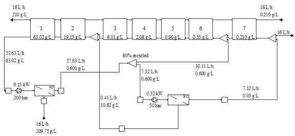
Figure 7. Simulation results for double pass configuration
