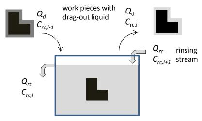
Figure 4. Input and output streams for a tank in the rinsing cascade
