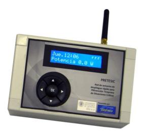
Figure 9. Detail of a QSDN node. Sensors are attached to it via connectors on the left side
