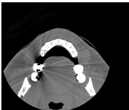
Figure 1: Example of MAR artifacts in a CT image from a jaw.
