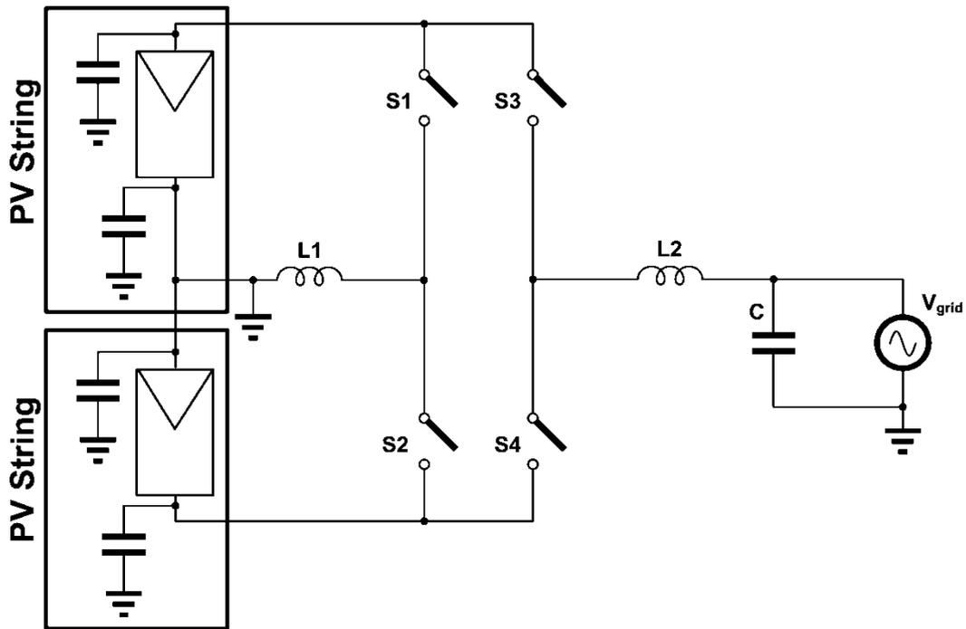
Fig. 8. The Half-bridge with generation control circuit topology.
