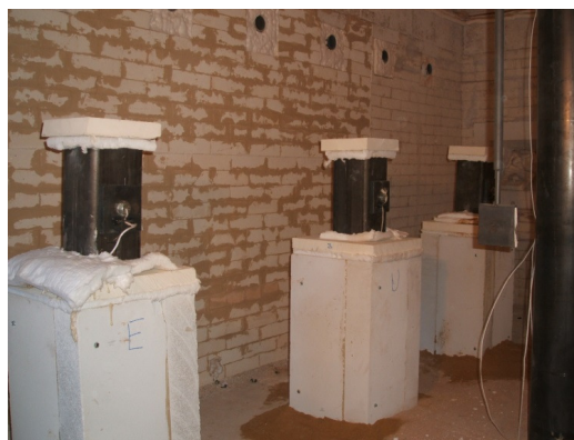
Figure 4.3. Location of test specimens in furnace [97]
