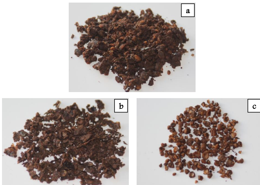
Fig. 3. Olive pomace (a) composed of pulps and peels (b) and pits (c).
