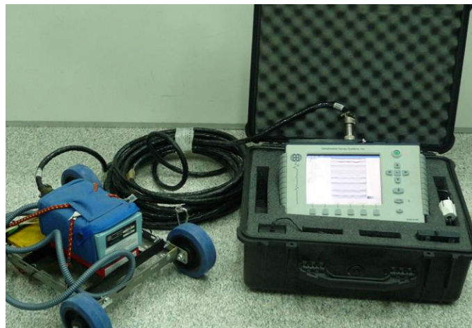
Figure 5.10. Picture of the GPR equipment used to scan the historical walls.
