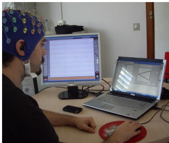
Figure 5.19. EEG capture process: a) spatial distribution of the 66 electrodes (10-10 system) for the capture of EEG signals; b) picture of one of the subjects undertaking the memory task. The electrodes are attached to the subject beforehand so they capture data during the memory task.
