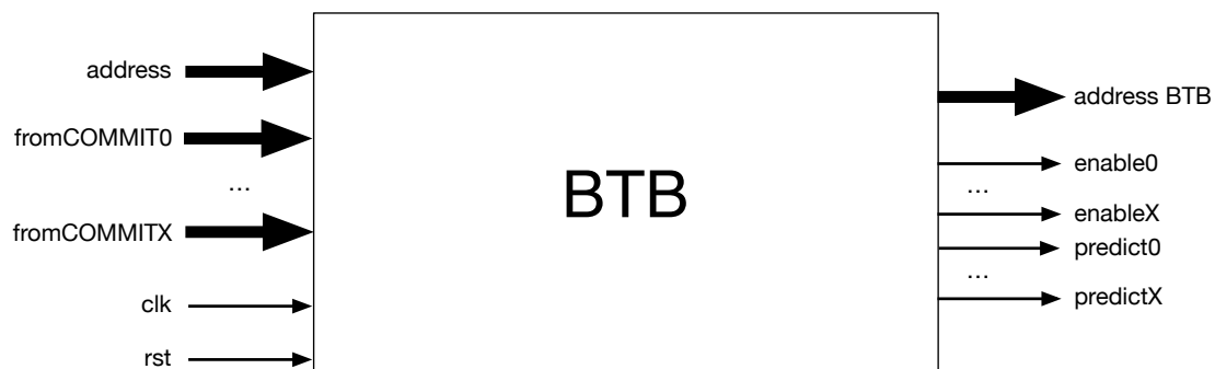
Figure 5.3: The connections to the BTB unit
