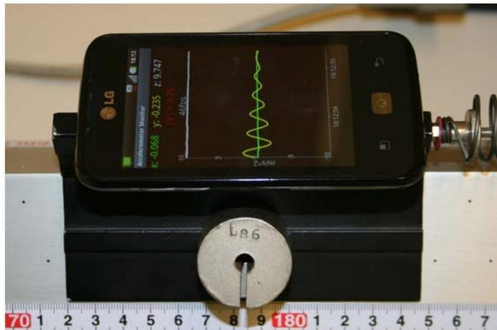
FIG. 5: Photograph of the smart phone displaying a view of the Acceleration Monitor application for the case of damped harmonic oscillations.
