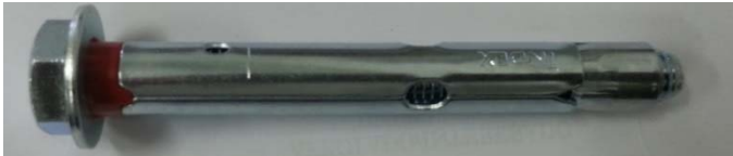
fig. 65 Tornillo Ø10mm L100mm Broca Ø12mm
