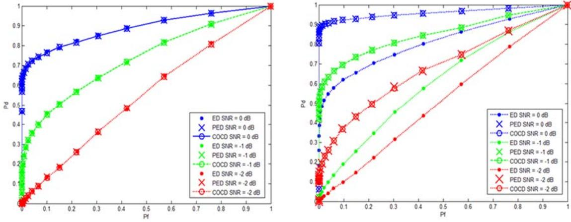
Figure 2. ROC curves: Independent Gaussian noise (left) and non-independent Gaussian noise (right)
