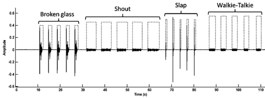
*Figure 1. Sequence of real acoustic events generated to verify the different detectors.*
