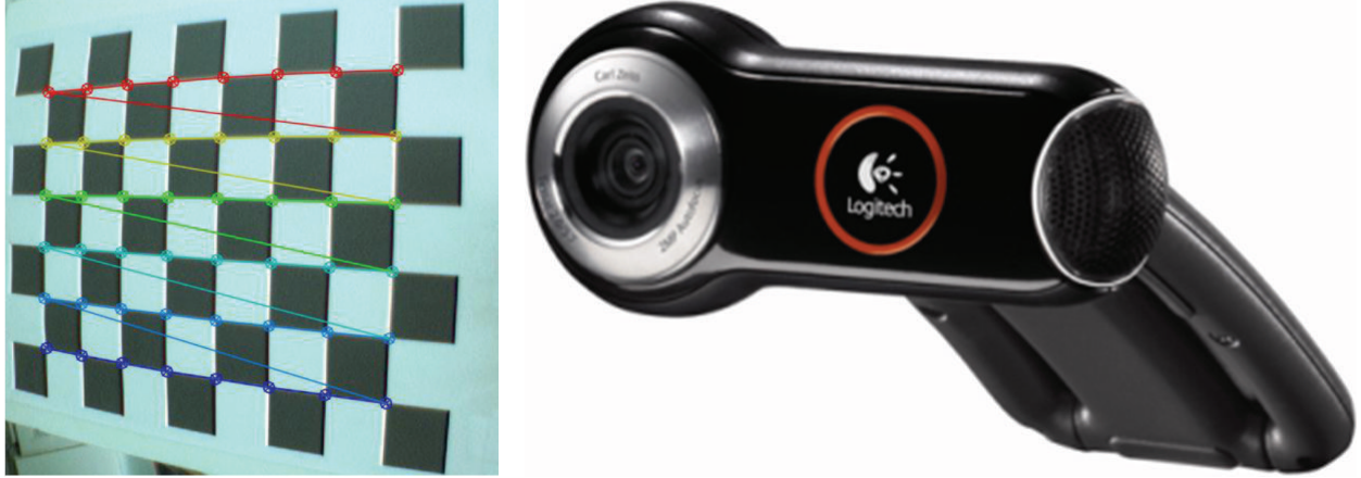
FIGURE 3: Checkerboard that is used to calibrate the camera. A Logitech QuickCam Pro 9000 webcam.
