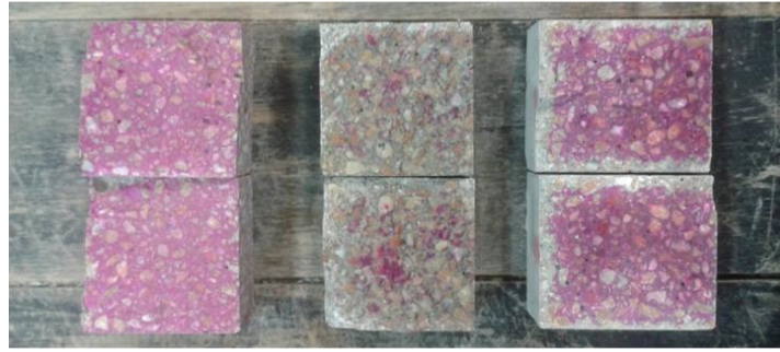
Figure 2. Application of the phenolphthalein indicator solution to a fresh fracture surface of concrete. From left to right C100*, C50-1-0 and C50-1-20.
