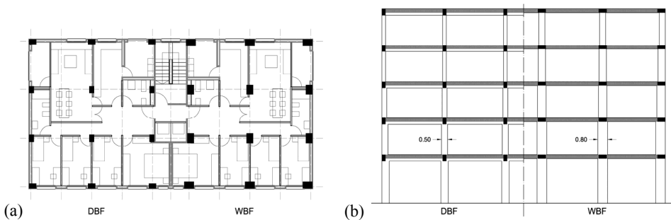
Figure 121: Distribution (a) and structural arrangement (b) of case-study version EC8 50-50 with DB and WB
