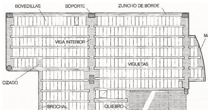
Figure 92: Typical wide-beam one-way joist slab system solution for common residential building (from De Andrés and CSCAE, 2009)
