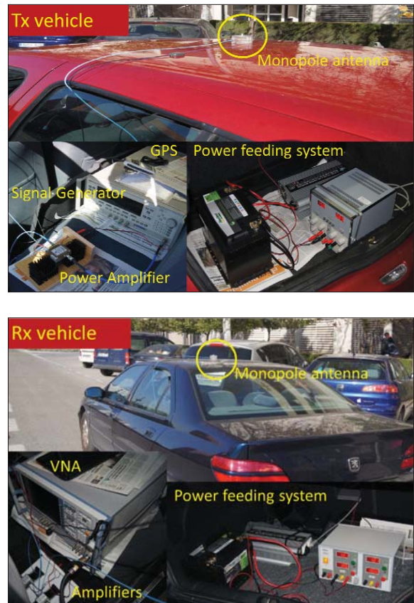
■ Figure 3. On board system setup: (a) Tx vehicle and (b) Rx vehicle.
