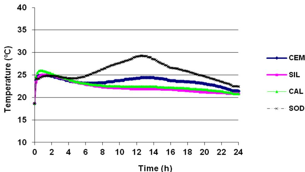
Figure 2. Hydration curves for mixtures of cement and SCSP with alkaline treatments.
