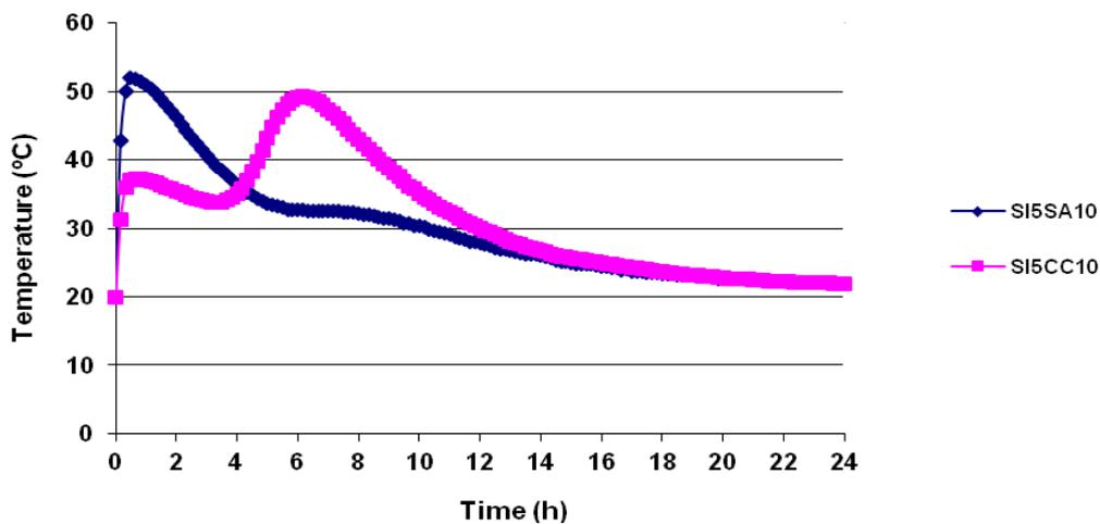
Figure 3. Effect of SCSP mineralization (dry mixture) on temperature evolution.
