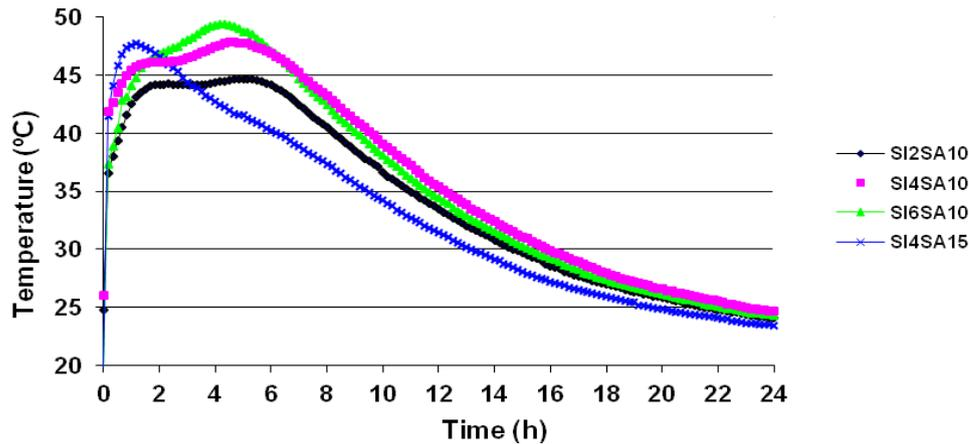
Figure 4. Effect of SCSP mineralization (wet mixture) on temperature evolution.
