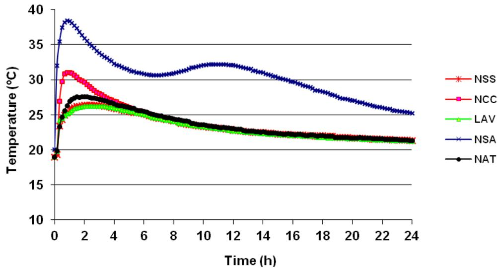
Figure 1. Hydration curves for natural SCSP and catalysts application on SCSP/cement mixtures.
