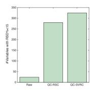
**Figure 2.** Number of variables showing  $RSD_{samples} < 15\%$  before and after correction of the intra-batch effect using QC-RSC and QC-SVRC. Note: Total number of variables in the data set = 552.
