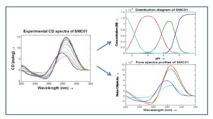
Figure 3. Experimental spectra of CD recorded throughout the acid-base titration of the SMC01 sequence. Pure spectra and proposed distribution diagrams obtained from EQUISPEC analysis.
