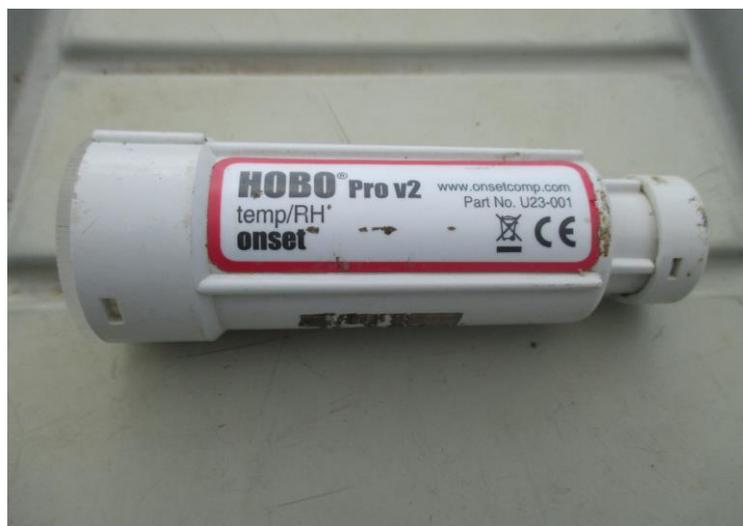
Figura 3: Data logger HOBO Pro v2.
