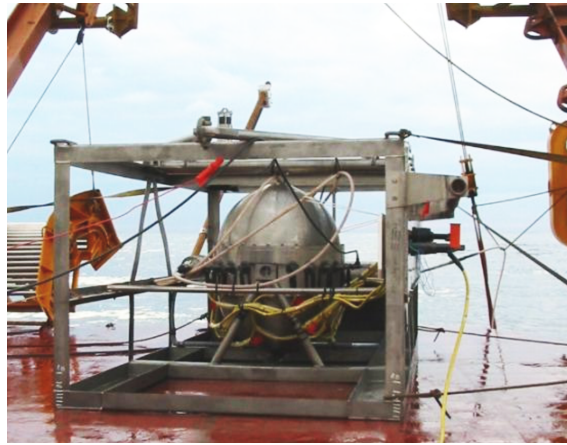
Figure 26: Junction box on the deck of the deployment ship.
