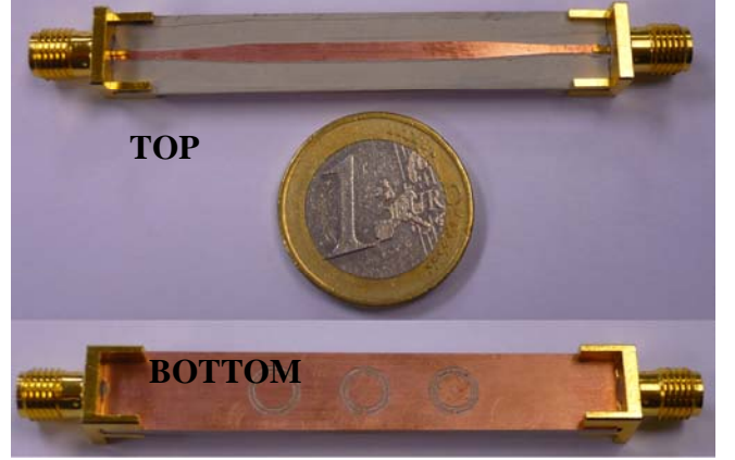
Fig. 12. Photograph of the fabricated CSRR-based stop-band filter.
