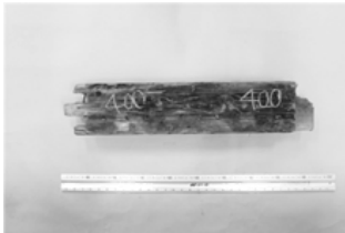
Photo5. Sample of salinized wood piece
