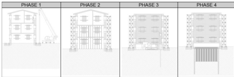
Figure 4. From the left: assembly of façade retaining structure, demolition of floor slabs, realization of the ground retaining system and excavation (when underground floors are required).
