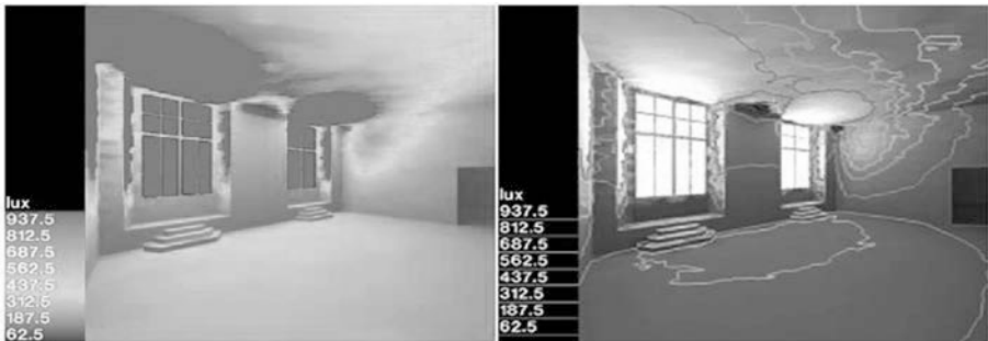
Figure 2 Example of Radiance simulations of "Sala del Terrazzo"
