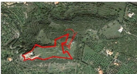
Fig. 11- Overlay mapping between the design (with a measurement scale that use roman palms) and a recent aerophotogrammetric survey.
