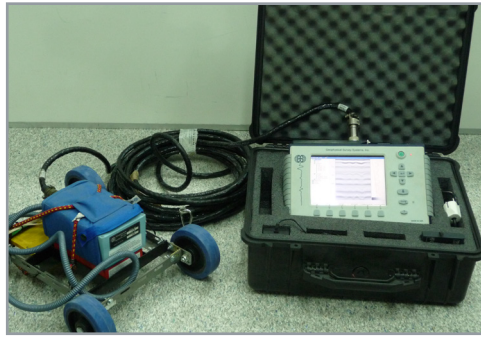
■ Figure 9. Photography of GPR SIR 3000 with 1.6GHz antenna plus displacement device
