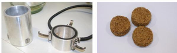
FIGURE 3. Left: Device used for measuring the flow resistance. Right: Samples prepared for the measurement.
