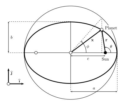
Figure 1: The geometry of the orbit of a planet.
