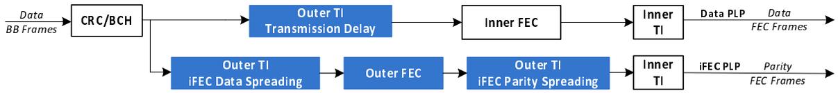
Fig. 1. BB-iFEC block diagram at the transmitter side, with two (inner and outer) FECs and TIs. The outer TI is divided in two (data and parity) spreading blocks. The iFEC physical layer pipe only transmits the parity generated by the Outer FEC, and it does not have an Inner FEC.
