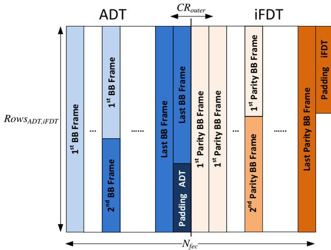
Fig. 4. BB-iFEC encoding matrix. ADT (Application Data Table) and iFDT (iFEC Data Table). The padding bits of the ADT are not transmitted. The padding bits of the iFDT can be used to transmit in-band L1 signalling.
