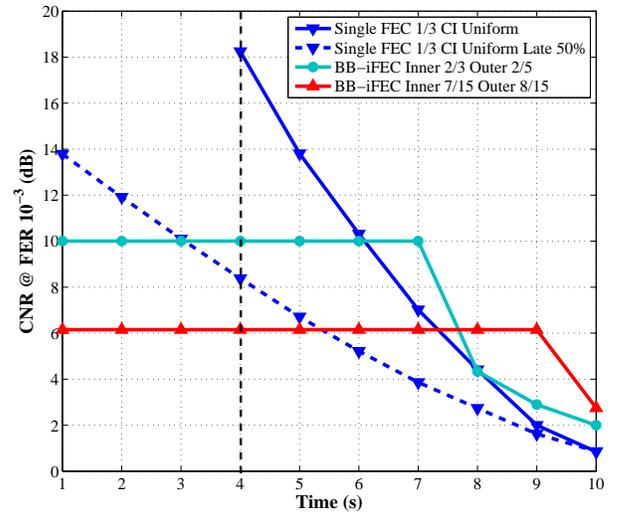
Fig. 9. Performance comparison between single FEC and BB-iFEC for an overall code rate  $CR$  1/3 in the TU6 channel at 10 Hz Doppler. Modulation is QPSK.
