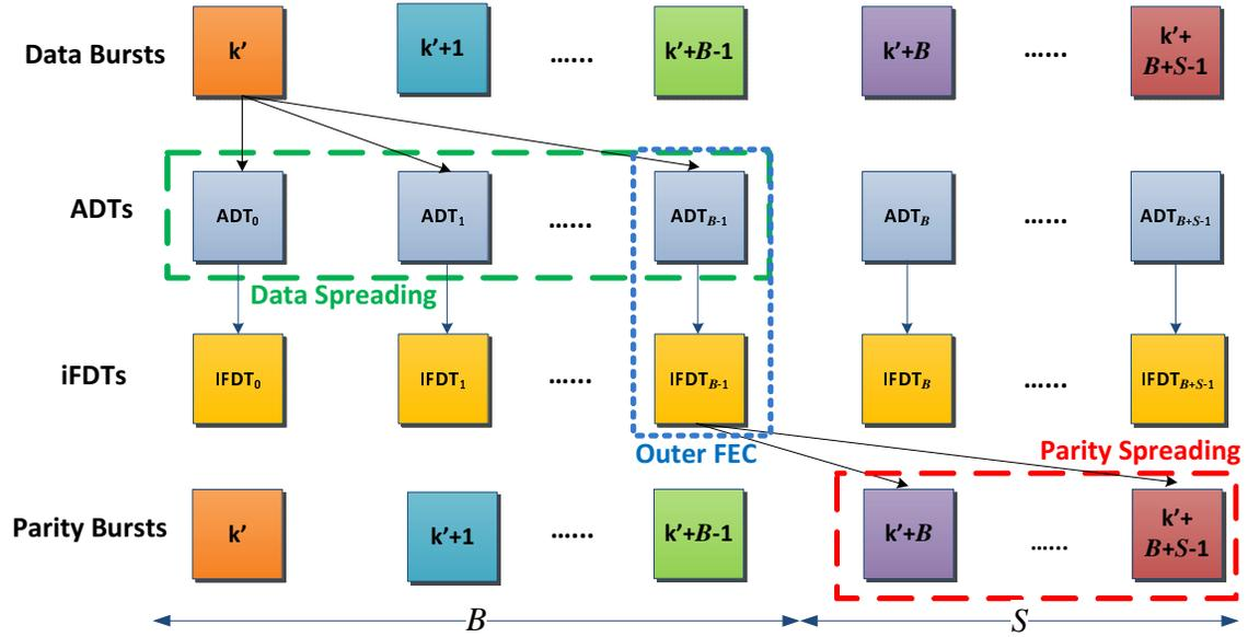
Fig. 2. Inter-burst interleaving with BB-iFEC with the parity transmitted after the data ( $D = 0$ ). The interleaving depth in number of interleaved bursts  $M$ , is equal to the data spreading factor,  $B$ , plus the parity spreading factor,  $S$ . After the generation of a parity burst, the data and parity spreading windows are shifted one element.
