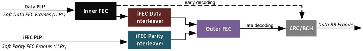
Fig. 6. BB-iFEC receiver block diagram. In early decoding mode the protection is given only by the Inner FEC. In late decoding mode the protection is given by both Inner FEC and Outer FEC.
