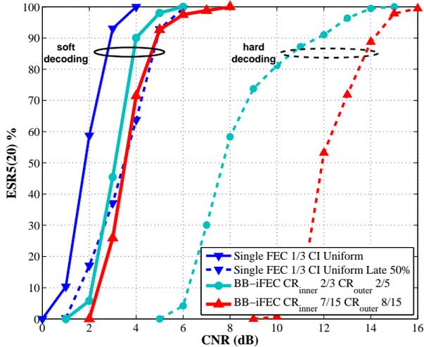
Fig. 8. Continuous performance comparison of single FEC  $CR$  1/3 and BB-iFEC ( $CR_{inner}$  2/3,  $CR_{outer}$  2/5) and ( $CR_{inner}$  7/15,  $CR_{outer}$  8/15) in the Sub-Urban (SU) LMS channel.
