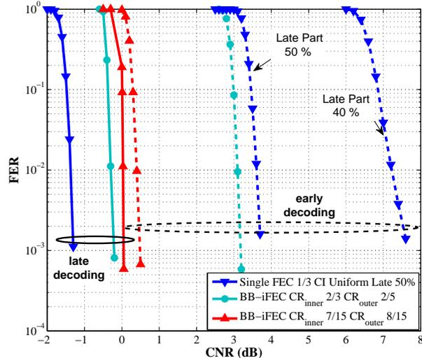
Fig. 7. Performance comparison between single FEC  $CR$  1/3 and soft BB-iFEC decoding ( $CR_{inner}$  2/3,  $CR_{outer}$  2/5) and ( $CR_{inner}$  7/15,  $CR_{outer}$  8/15) in the AWGN channel. Modulation is QPSK.
