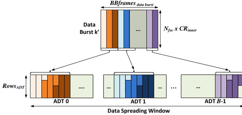
Fig. 3. Illustration of the data spreading process. The data spreading process is performed from one data burst to  $B$  ADTs (Application Data Tables). The parity spreading process is performed from one iFDT (iFEC Data Table) to  $S$  parity bursts. Each ADT/parity burst contains an entire number of consecutive BB frames of the data burst/iFDT. The maximum difference between ADTs/parity bursts is one BB frame.
