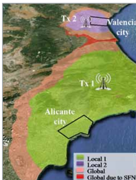
■ Figure 11. Coverage area for global and local services in Valencia community (Spain).
