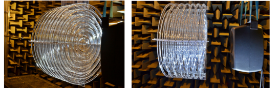
FIG. 3. (Color online) Views of the experimental set-up showing the lens-source system.
