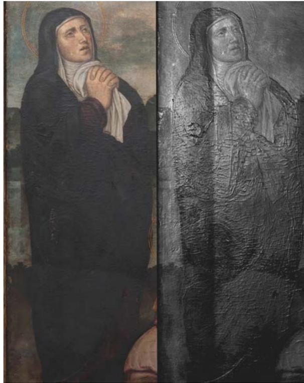
**Fig. 5.** Detail panel painting “El Calvario”, visualized in RTI with flat light (left) and specular enhancement (right). RTI offers a clearer and more detailed view of the wood support deformation, and the cracking, scratching, losses, and cupping of pictorial layers.
