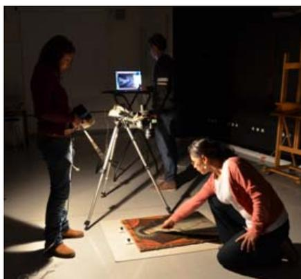
**Fig. 2.** Conservators during data capture using the RTI Highlight method, where a light source is moved around the object and a new image is taken for each light angle.
