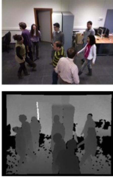
Figure 2: Examples of aligned RGB and depth images obtained with kinect.
