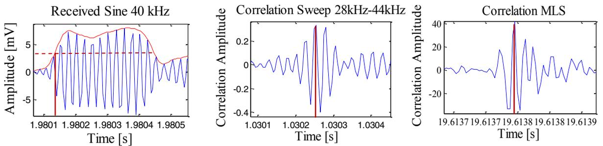
Fig.2 Examples of: received sine signal of 40 kHz with envelope (left), cross-correlation of received sine sweep signal from 28 kHz to 44 kHz (middle) and cross-correlation of received MLS signal (right).
