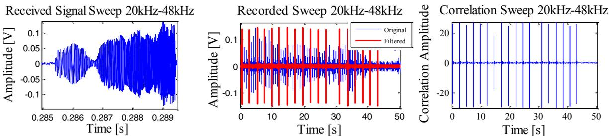
Fig.3 Example of sine sweep signal from 20 kHz to 48 kHz: a single received (left), recorded (middle) and correlation (right).
