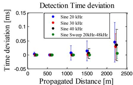
Fig.6 Values of deviation time (mean and sigma), with respect the true time, for the detected propagated signal with noise. It is determined by the correlation detection method.
