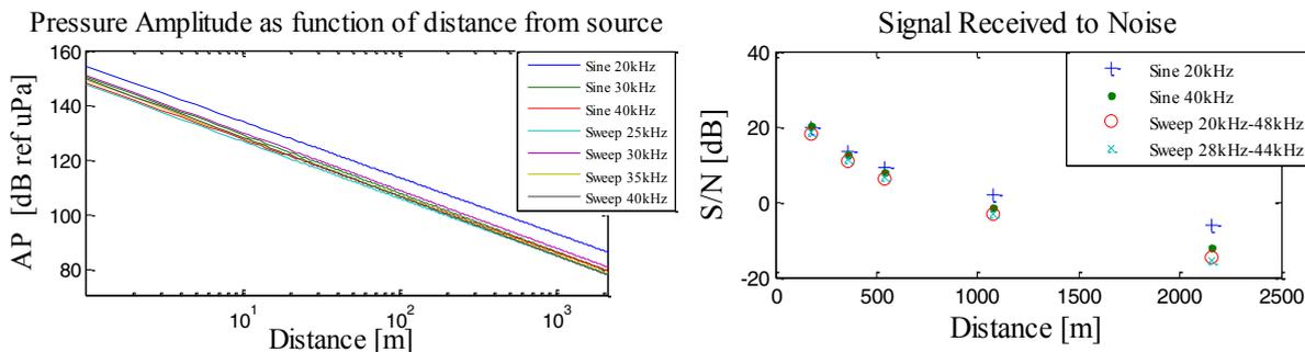
Fig.5 Pressure amplitude emitted by the acoustic transmitter FFR SX30+SEB per distance (left). On the right, the signal to noise ratio (dB) per signal under sea water conditions of ANTARES site.
