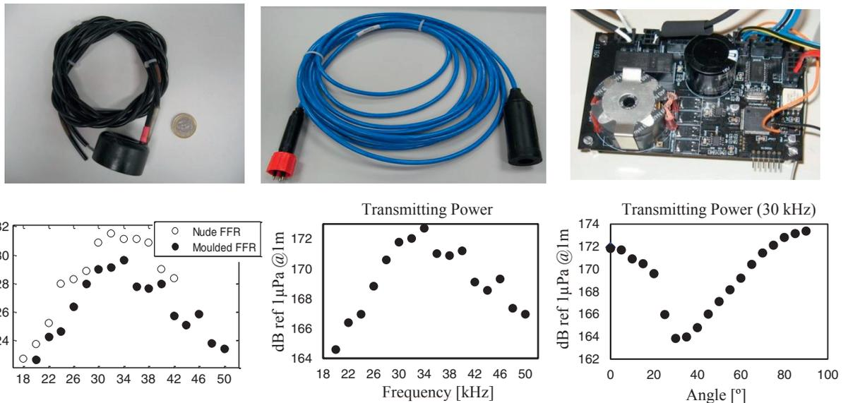
Fig.1 On top, view of the Free Flooded Ring transducer without over-moulding (left) and with (middle) and the Sound Emission Board (right). On bottom, Transmitting Voltage Response of the transducer in function of frequency (left), Transmitting Power (versus frequency in middle and versus angle in right).
