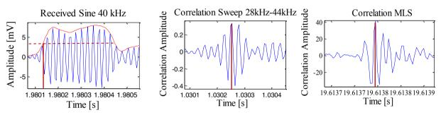
Fig.2 Examples of: received sine signal of 40 kHz with envelope (left), cross-correlation of received sine sweep signal from 28 kHz to 44 kHz (middle) and cross-correlation of received MLS signal (right).
