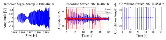
Fig.3 Example of sine sweep signal from 20 kHz to 48 kHz: a single received (left), recorded (middle) and correlation (right).
