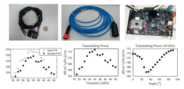
Fig.1 On top, view of the Free Flooded Ring transducer without over-moulding (left) and with (middle) and the Sound Emission Board (right). On bottom, Transmitting Voltage Response of the transducer in function of frequency (left), Transmitting Power (versus frequency in middle and versus angle in right).
