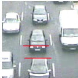
d) User presses space key the third time to indicate that the vehicle's tail has exceeded the main line and the annotation of the (first) vehicle has just finished. (frame 10568).
