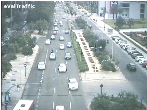
Figure 2. Setting the locations where to perform the measurements
