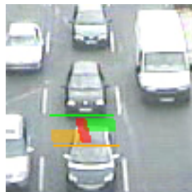
d) User presses space key the third time to indicate that the vehicle's tail has exceeded the main line and the annotation of the (first) vehicle has just finished. (frame 10568).
