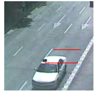
d) User presses key the third time to indicate that the vehicle has exceeded the main line and the annotation of the vehicle concludes, returning to the initial state.
