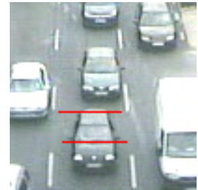
g) User goes forward until the (second) vehicle reaches the main line and then presses space key. h) Finally, the space key is pressed to mark the rear part of the (second) vehicle on the main line.
