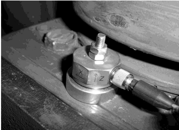
Fig. 2. Detail of bogie mounted accelerometer with oriented axes
