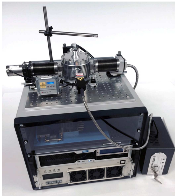
Fig. 3. Photograph of the manufactured dual mode microwave cavity.
