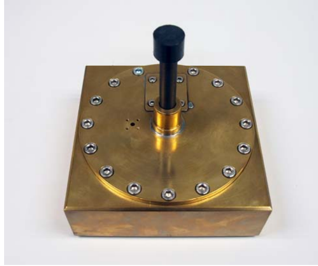
Fig. 4. Cylindrical cavity used to measure a ROD of dielectric material ( h=40 mm; R=51.917 mm; b=6.325 mm; a=6.250 mm; \epsilon_2=\epsilon_3=1 )
