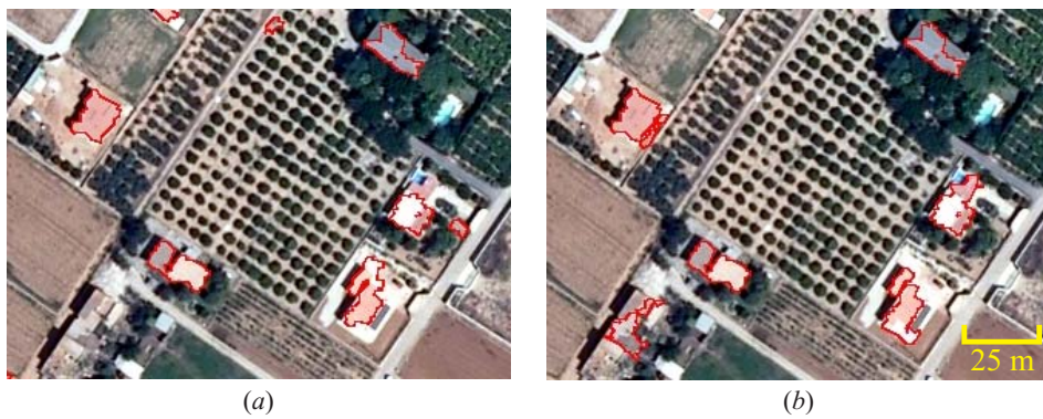
Figure 4: A detail of the building classification contours shown over the 2007 scene using RGB bands in (a) and using RGB and SAR bands in (b).
