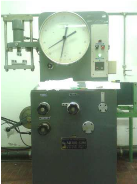
Figure 3.18- Hydraulic press METROCOM
